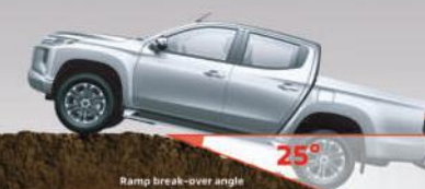
Ramp Break-over Angle
