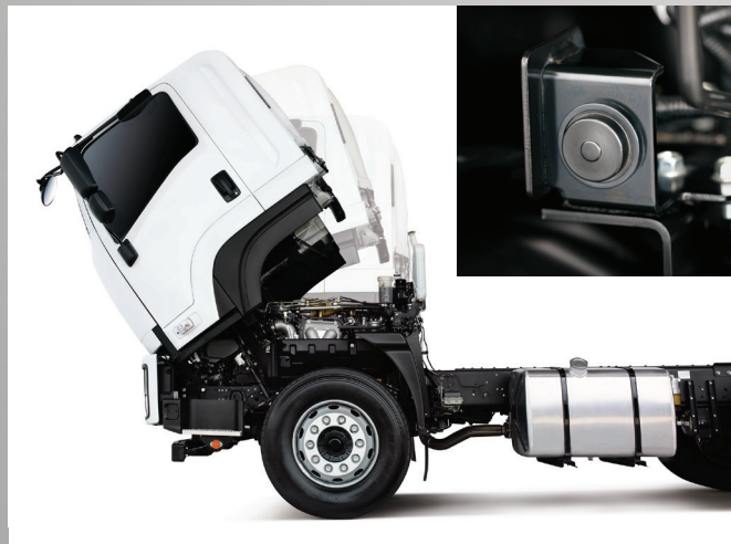
▼ Electric driven hydraulic cab tilt.
