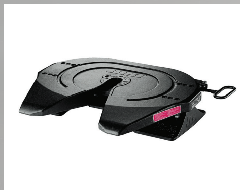
▲ Ancillary fitting includes JOST cast Fifth Wheel, Susie Hose, Step Platform and Parlok Rigid Mudguard.
