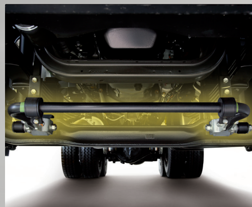
▲ Stabiliser Bar (Applicable to FXZ77UU-M).
