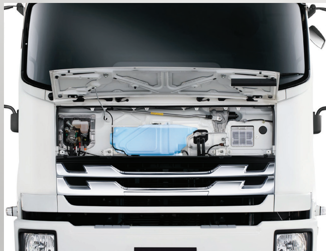
▼ Quick access panel. Designed for convenience, inspecting or replacing clutch fluid, wiper fluid and cabin air filter can be done quickly and safely.
