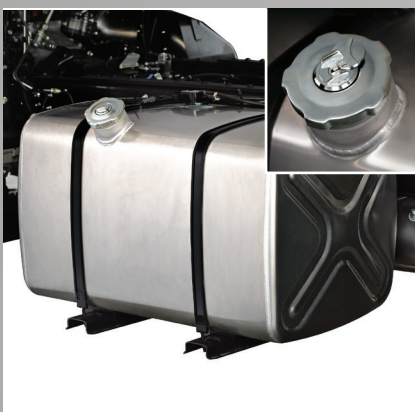
▲ Bigger and durable aluminium alloy fuel tank with lockable cap.
