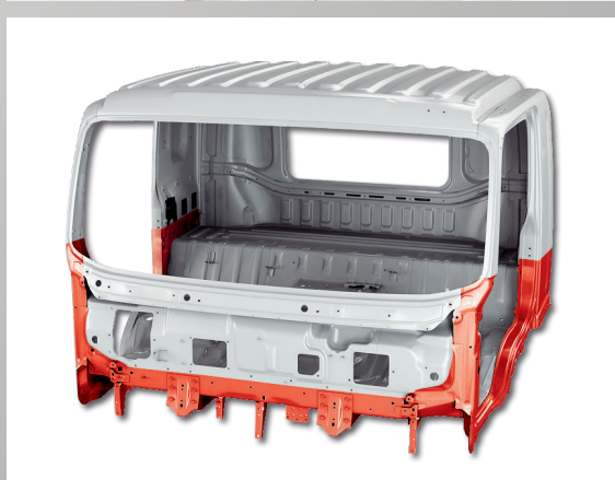
▲ High rigidity cab with cation electrodeposition coating.
