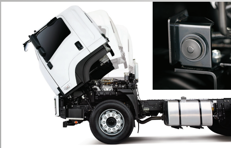
▼ Electric driven hydraulic cab tilt.
